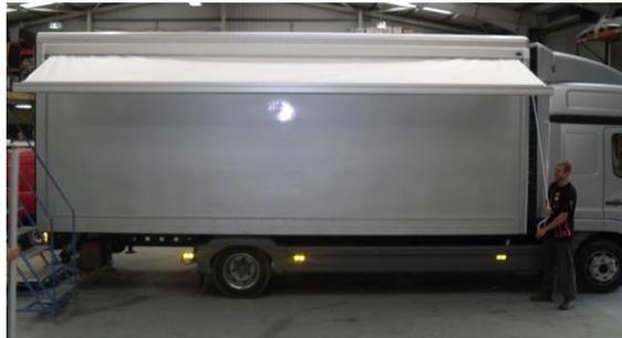
**Note** – when winding out the roof you will need to support the fascia especially on the larger models.
