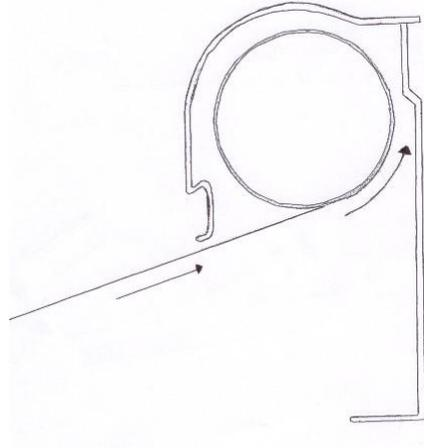
Check that the roof sheet pockets have not folded over – this can cause the fascia not to close on one side.
