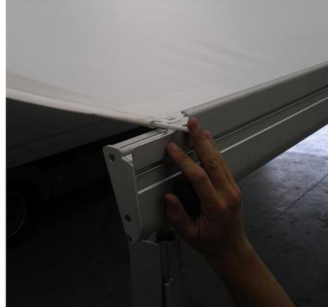
Take side awning rail section, these are not handed; they can be supplied joined for storage purposes, make sure they are solid when fitting.
