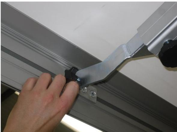
Now secure at the fascia end with hand wheel, the bar is at a tight angle when doing this so you will need to slide it into position from the left hand side over the fascia bracket and fasten.
