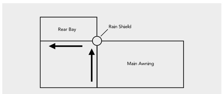
2. Whilst the roof sheet is still in a folded/rolled position, slide one side up the top slot in the roof rail of the main awning.
