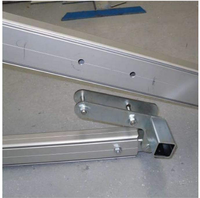
The roof rail is connected to corner post and secured using the 17mm spanners, this assembly is carried out with the parts still on the floor, repeat for each post.
