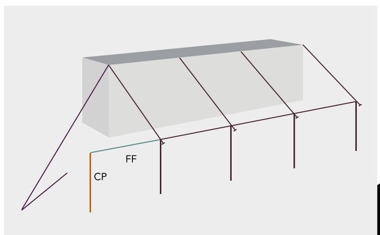
4. Attach the corner post to the diagonal rail and lift into position. Again ensure that one person supports this post. We recommend that you fix this post to the floor.
