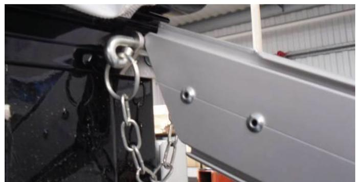
The roof rail is now allowed to slope down and rest on the floor. This operation is now repeated for the remaining roof rails along the main structure.
