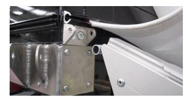
The roof rail is now allowed to slope down and rest on the floor. This operation is now repeated for the remaining roof rails along the main structure.
