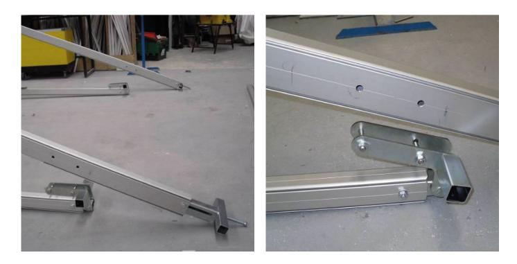
The roof rail is connected to corner post and secured using the 17mm spanners, this assembly is carried out with the parts still on the floor, repeat for each post.
